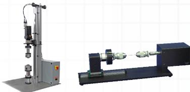
ADMET torsion testing systems are configured in either a vertical or horizontal orientation. These systems employ a linear slide design for maximum torsional stiffness and minimal axial friction. All torsion systems feature unlimited rotation in both directions and are ordered in either horizontal or vertical orientation.
